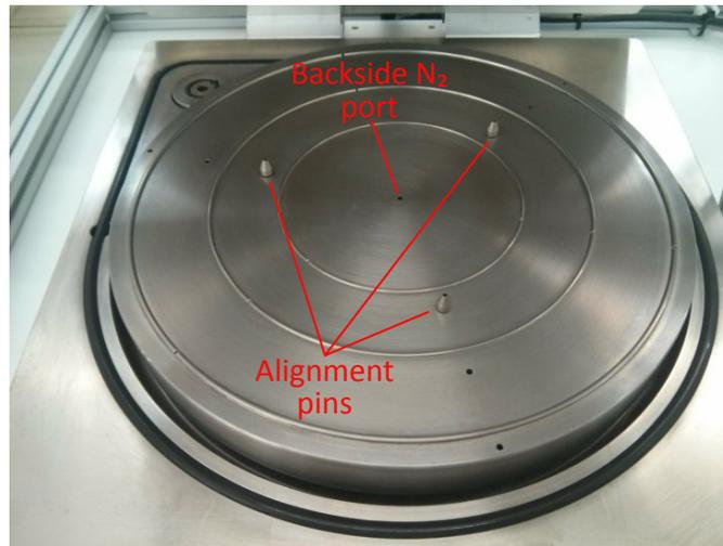
Figure 2: Sample chuck: single backside N<sub>2</sub> port and wafer pins
