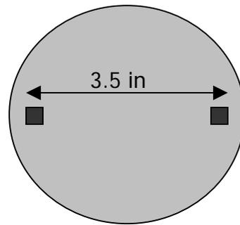
Alignment marks should be placed near the edge and along the centerline of the substrate, ex. on a 4 in silicon wafer.
