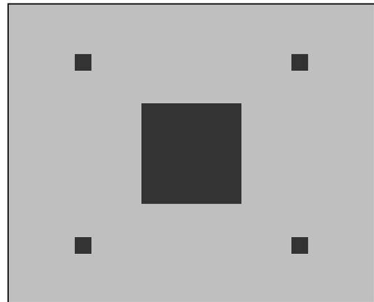
Mask 4. This mask will have a longer write time compared to Mask 2, however it will be much shorter than Masks 1 and 3. The pattern generator only writes where it has to, and because the design is not outlined, it can skip over the areas with nothing in it.
