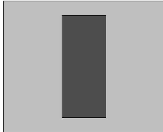
Mask 6. Optimization of this design allows the pattern generator to skip over the blank areas to the left and right of the design. This will significantly decrease the write time.
