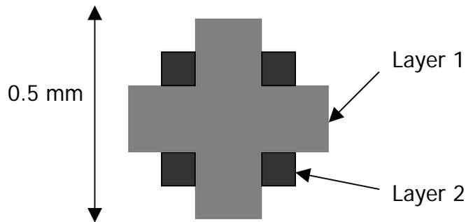
Typical alignment marks for a 2-layer mask where the cross is layer 1 and the squares are layer 2.
