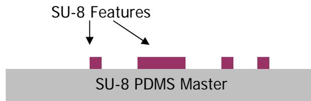
Fig 1. Side view of a SU-8 PDMS master. Because of the difficulty removing PDMS, the photoresist remain on the master and becomes the features. Note: drawing not to scale.
