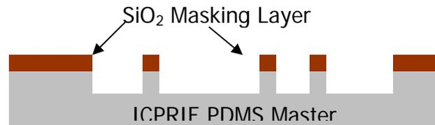
Figure 2. Side profile of an ICPRIE PDMS master. The silicon dioxide layer resists the plasma etch while the exposed silicon does not.
