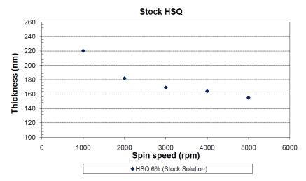
Figure 1 Spin curve for stock 6% HSQ (constant 2 sec ramp time)
