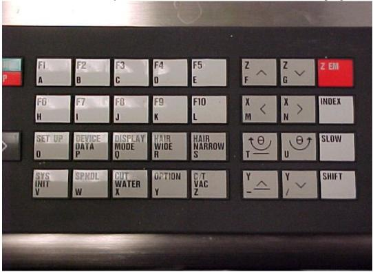
15. Choose a line that runs across the width of the substrate (or two features that are even). Using the movement keys, align to the three dashed lines across the screen.
