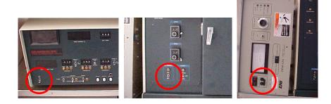
3.1.2 Once the chamber reaches its base pressure of <200mT, the alarm will sound; press the Reset button to turn off the alarm and vent the chamber.
